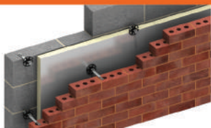
Block & Brick Cavity Wall Insulation
